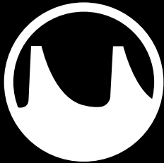
CONVENTIONAL 'BUTTRESS' THREAD FORM
