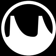
CONVENTIONAL 'BUTTRESS' THREAD FORM
